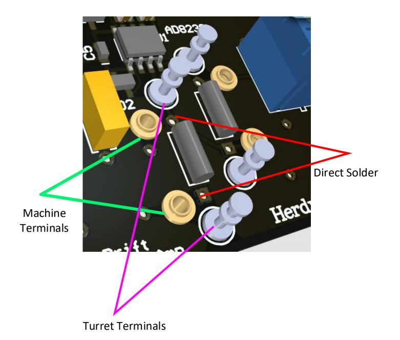
Gain Programming resistors may be installed via direct-solder, push-in machine terminals, or wrap-around turret terminals.
