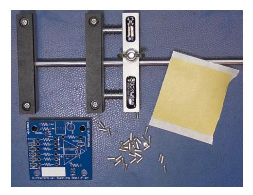
2. Place the terminals into the PCB from the top.
