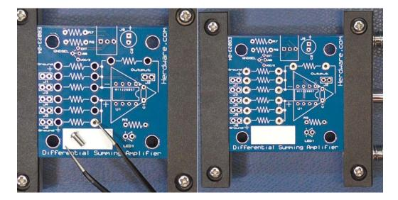
3. Once the terminals are all inserted into the PCB, peel the backing and apply the included 2" square piece of tape to hold the terminals flush while soldering.
