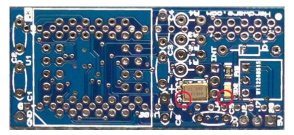
These parts can be soldered with a regular soldering iron but it is easier to use solder paste and a hot air solder station. The kit is available with these three parts already assembled.
