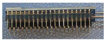
6. You may choose to clip the pins on the top underneath the 44 Pin socket and the 10 Pin programmer header. I found that this wasn't really necessary if the solder joints are clean. (Rev 2 board shown as example)
