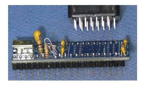
8. Likewise solder the 10 Pin header, the two 3 pin header and the right angle 3 pin connector. Sometimes it helps to grab a pin from the top of the PCB with needlenose pliers long enough to tack a pin.
