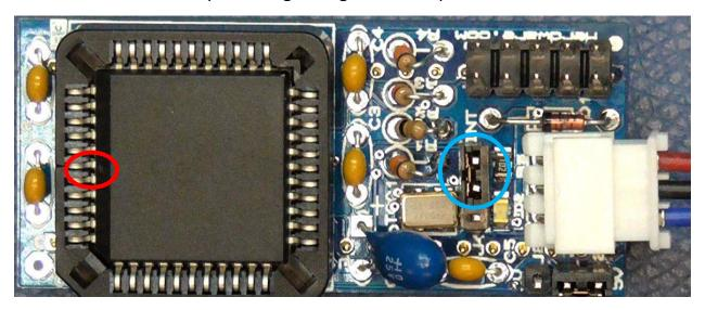
9. Insert the 44 Pin PLCC carefully into the socket taking note of the bevel (green circle) and the pin 1 dot (red circle). Put the jumper on the 3 pin header as shown below (blue circle) to select the onboard oscillator.
