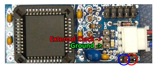
11. To use the Herdware 3 Pin Connector to supply and select between +3.3V and +5V plug the connector in and supply +5V on the Red wire and/or +3.3V on the Blue while the Black wire is ground.
